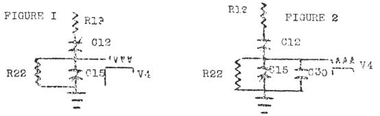
Note than R19 and C12 are in series with R22 and C15 which are in parallel. This is the basic positive feedback loop of a Wien Bridge.
